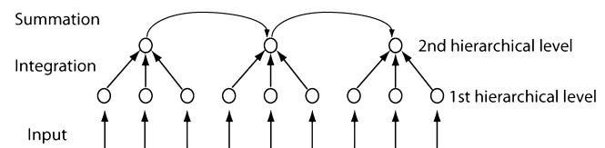
**Fig. 1.** Schematic representation of the integrative neural model. The first hierarchical level receives the input per pixel and performs the integration of each of the three inputs in a “three to one” way. Afterwards, the result is transmitted to the second hierarchical level where further integration is performed by the cumulative summation of the first-level values.
